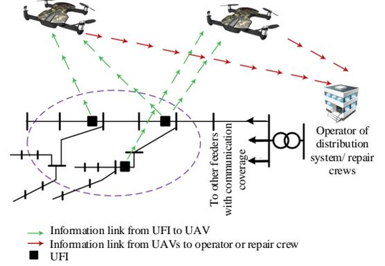
(b) UFI-UAV and UAV-operator links
