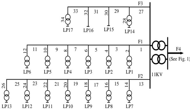
Fig. 3: Feeders 1, 2, and 3 of the test system located in the areas with acceptable communication coverage [32].
