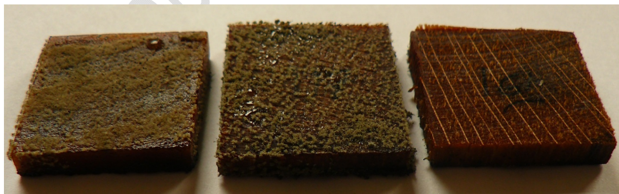
111 Figure 1. Beech wood samples impregnated with olive oil (left), fennel oil (centre) and lemon 112 grass oil (right) incubated with Aspergillus niger .
